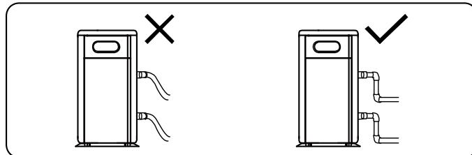
2) In order to guarantee the heating efficiency, the water pipe length should be ≤10m between the pool and the heat pump.
